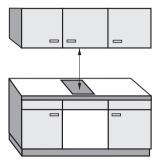
If there is more than one appliance beneath a hood (e.g. wok burner and electric combiset), and they have different minimum safety distances always observe the greater distance.
